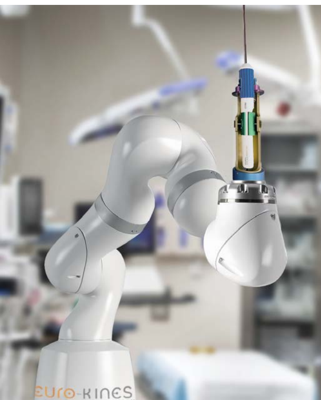
The Proteus™ II Robotic Arm is shown here holding the Huygens™ Catheter handle with a short version of the Huygens™ Catheter as initial control testing of the Gripper's ability to control axial control and tip deflection is done.
