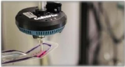
Our Predator3D™ product line performs error-proofing of the dispensing of sealants and structural adhesives. It is primarily used for structural adhesive bead volume and location in body assembly and room temperature vulcanization, used for sealing in engine and transmission assemblies.
